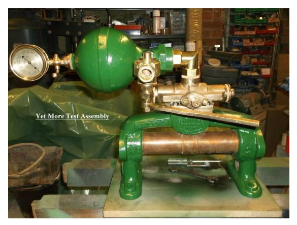
At various stages the restored or remanufactured parts were fitted back together to ensure the fit and relation of everything was right.
