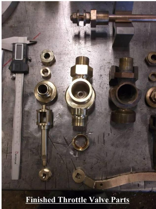
Finished Throttle Valve Parts
