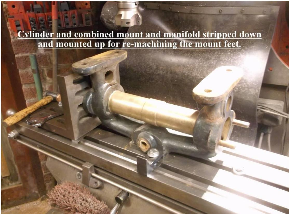
Cylinder and combined mount and manifold stripped down and mounted up for re-machining the mount feet.
