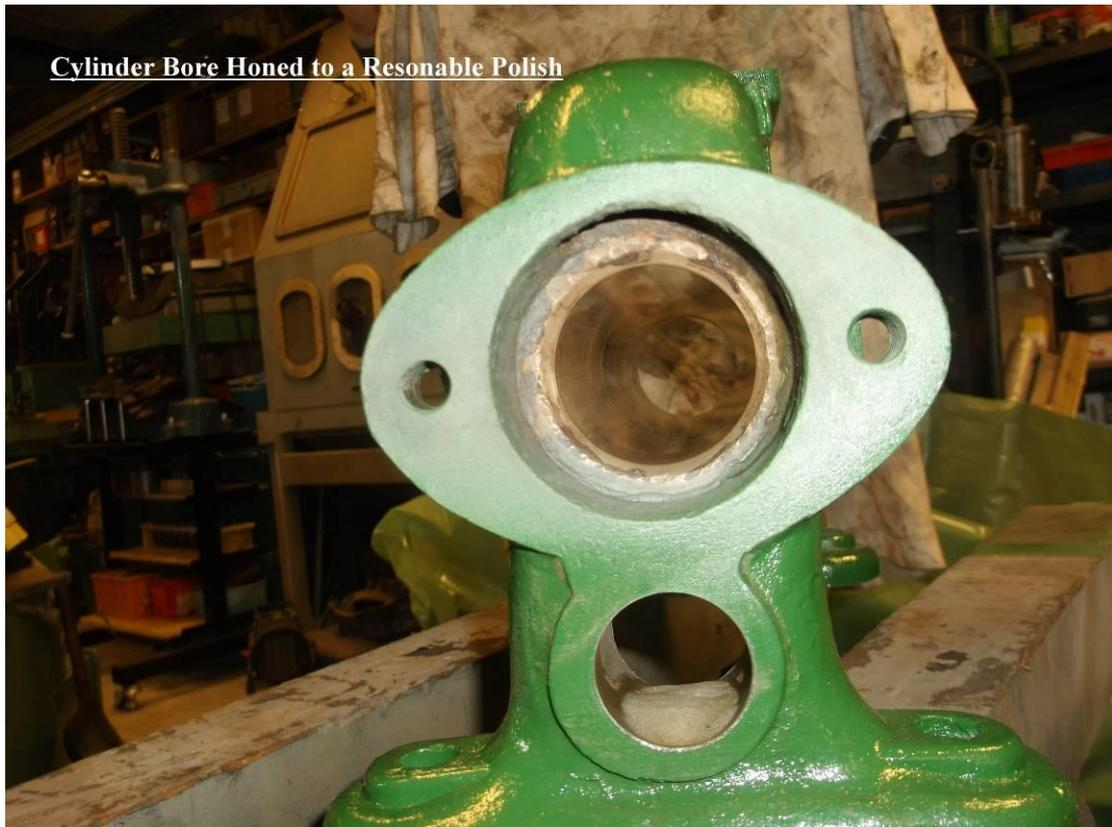
Cylinder studs, nuts and those for the valve chest were all remade in stainless steel. The valve plate and any mating machined surfaces were all remachined flat and true.
